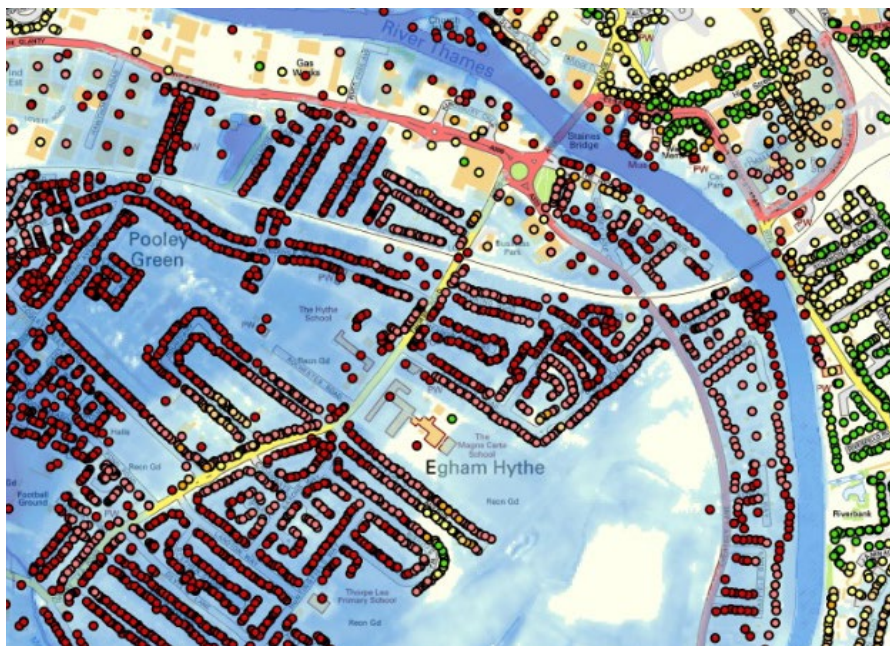
Visualisation of the underlying data to FloodScore; showing Ambiental UKFloodMap4™ overlay with OS AddressBase building points, colour classified depending on their FloodScore value.
